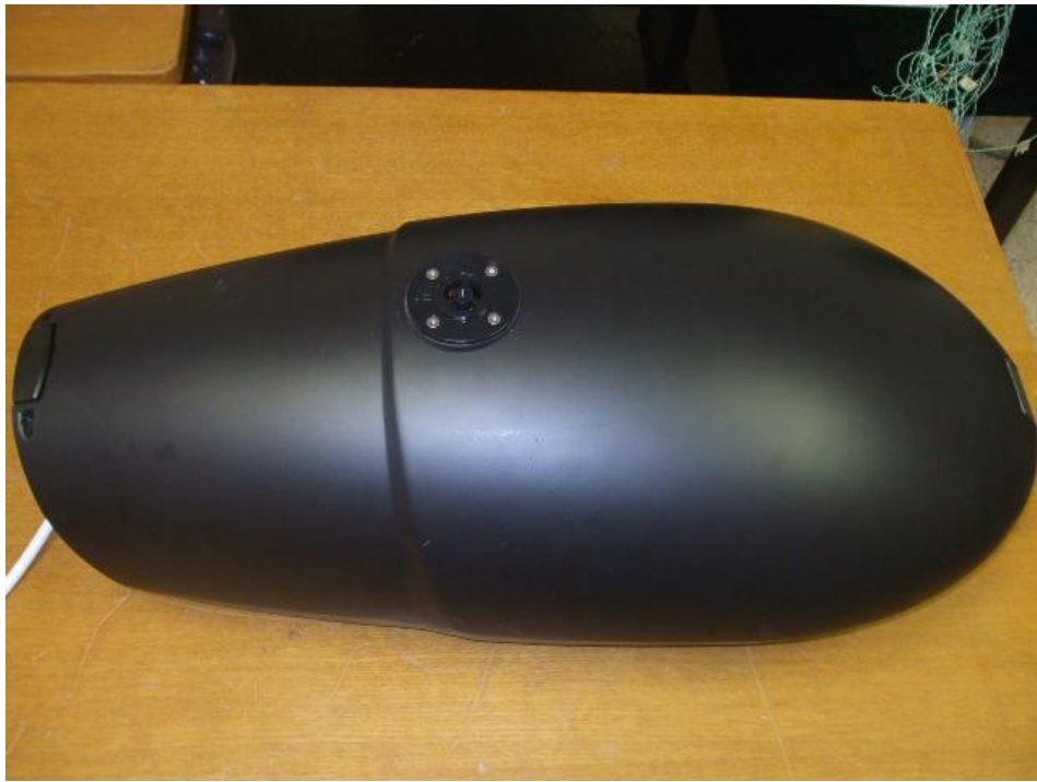
Sample street lamp enclosure
